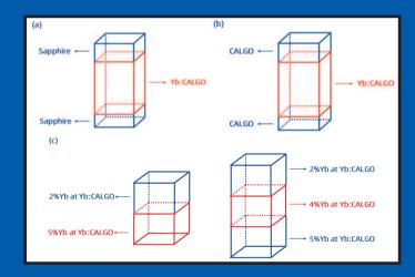
Crylink's Yb:CALGO crystals are routinely designed as dual-pass facet-coated cubes or disks. These can be combined with a front-end LD pump module or a front-stage mode-locked system to achieve laser outputs with pulse widths within 100 femtoseconds.
